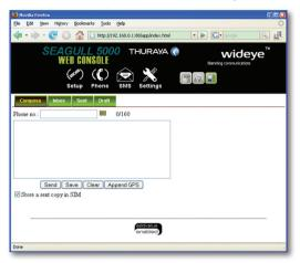
4.2.2 To send the TEXT message, enter the recipient's phone number in the following format: <+><Country code><Telephone number> and click the **Send** button. If the TEXT message requires GPS information, click the **Append GPS** button to append the GPS location to the TEXT message prior to sending.
